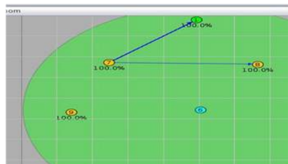
Figure 1 : WSN configuration without the malicious node after starting the simulation.
