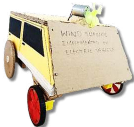
Figure 2: Prototype of Electric vehicle with wind turbine
