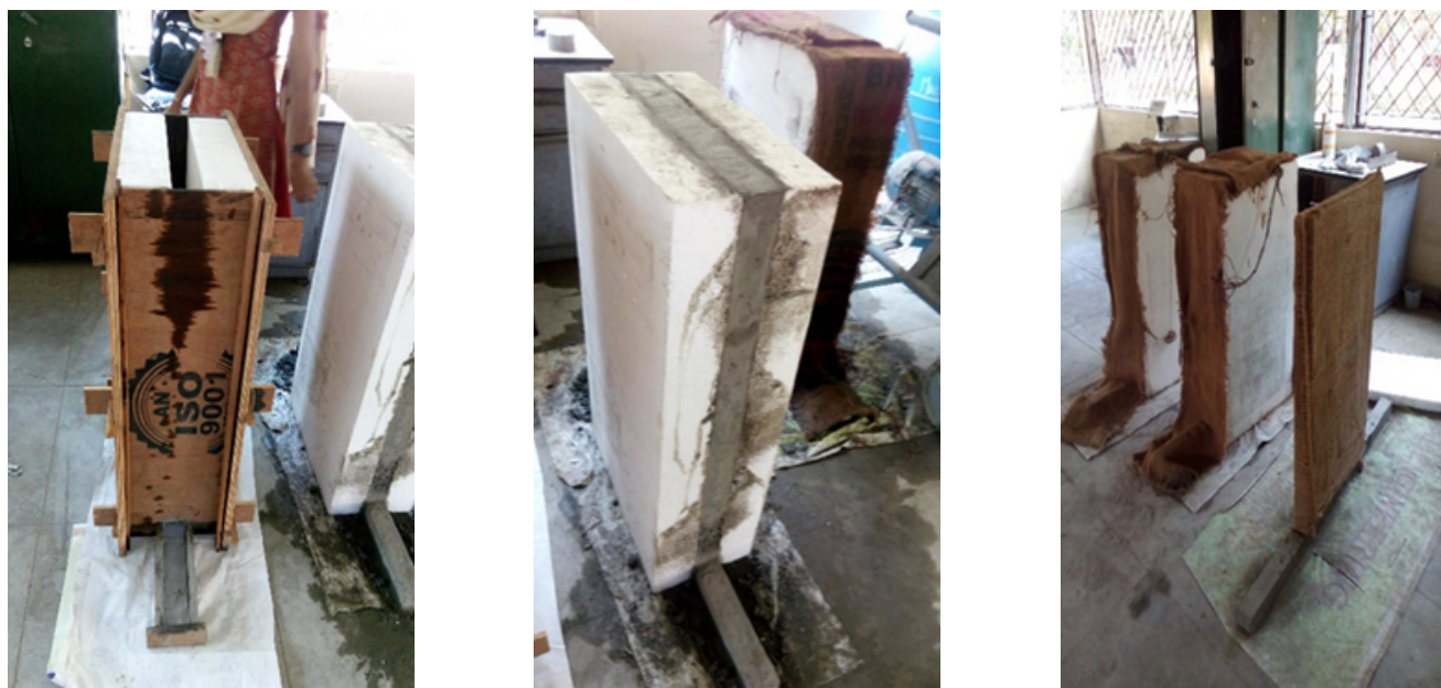
Fig 1. Typical cast specimens of ICF wall panels with plain concrete panel
