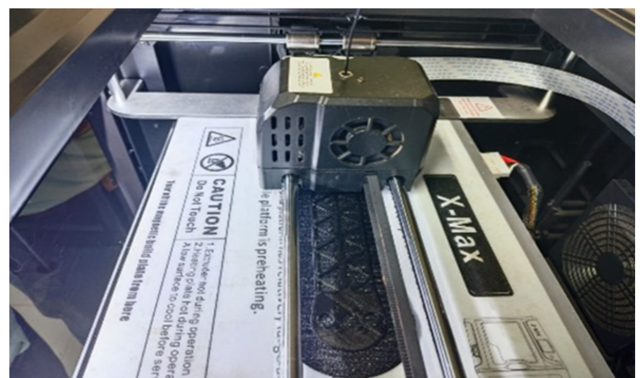
Fig 5. 3D printing of the drone wing
